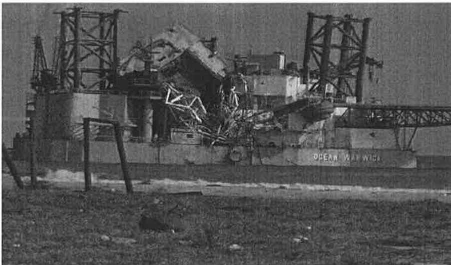
Hurricane Katrina caused the Ocean Warwick Drilling Rig to 'beach' on Dauphin Island after drifting 66 nautical miles from its drilling location.
